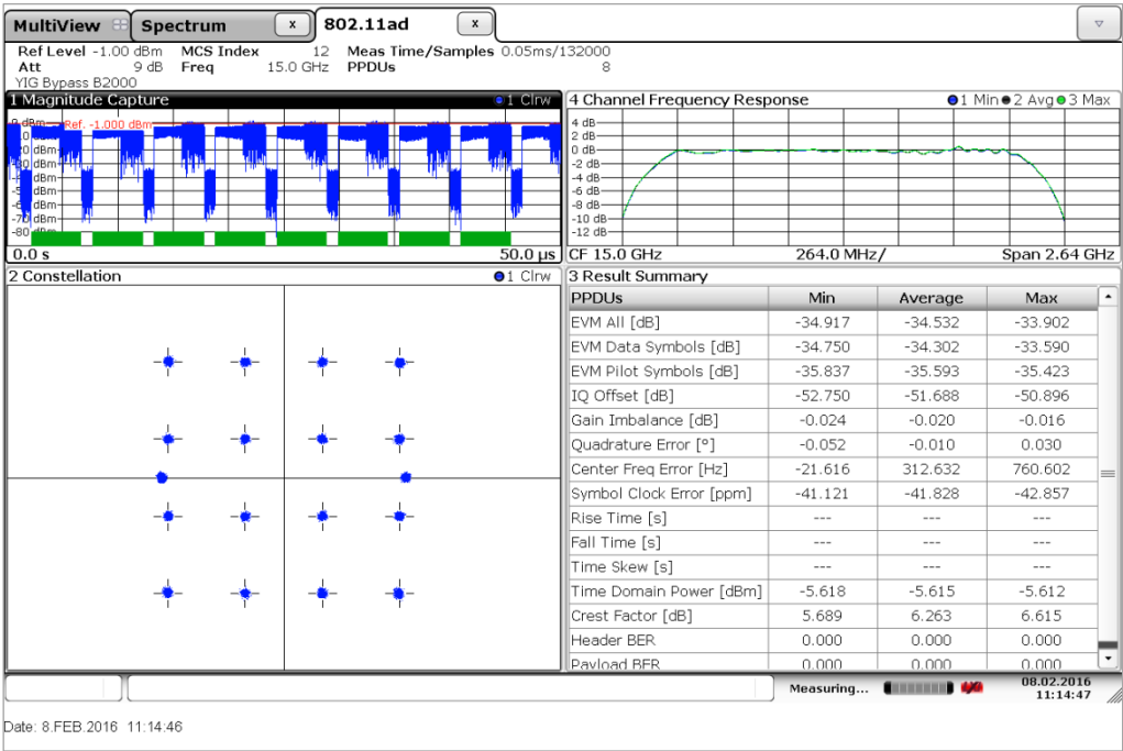
Measured EVM for an IEEE 802.11ad signal with 1.76 GHz bandwidth (MCS12, at 15 GHz IF)
